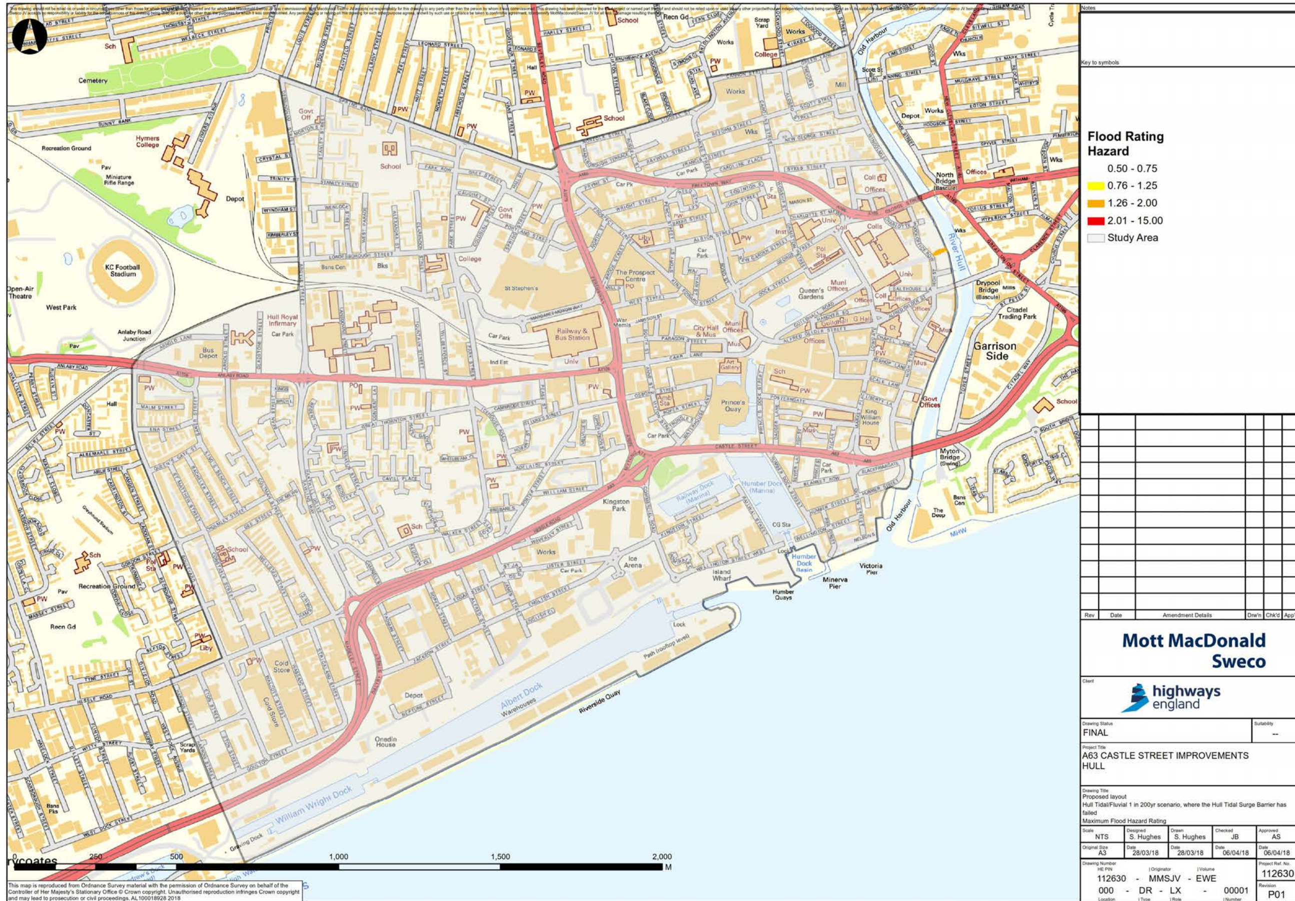
Figure 13.58 1 in 200-year River Hull tidal / fluvial flooding maximum flood hazard rating for Scheme layout (Hull Tidal Surge Barrier open)
