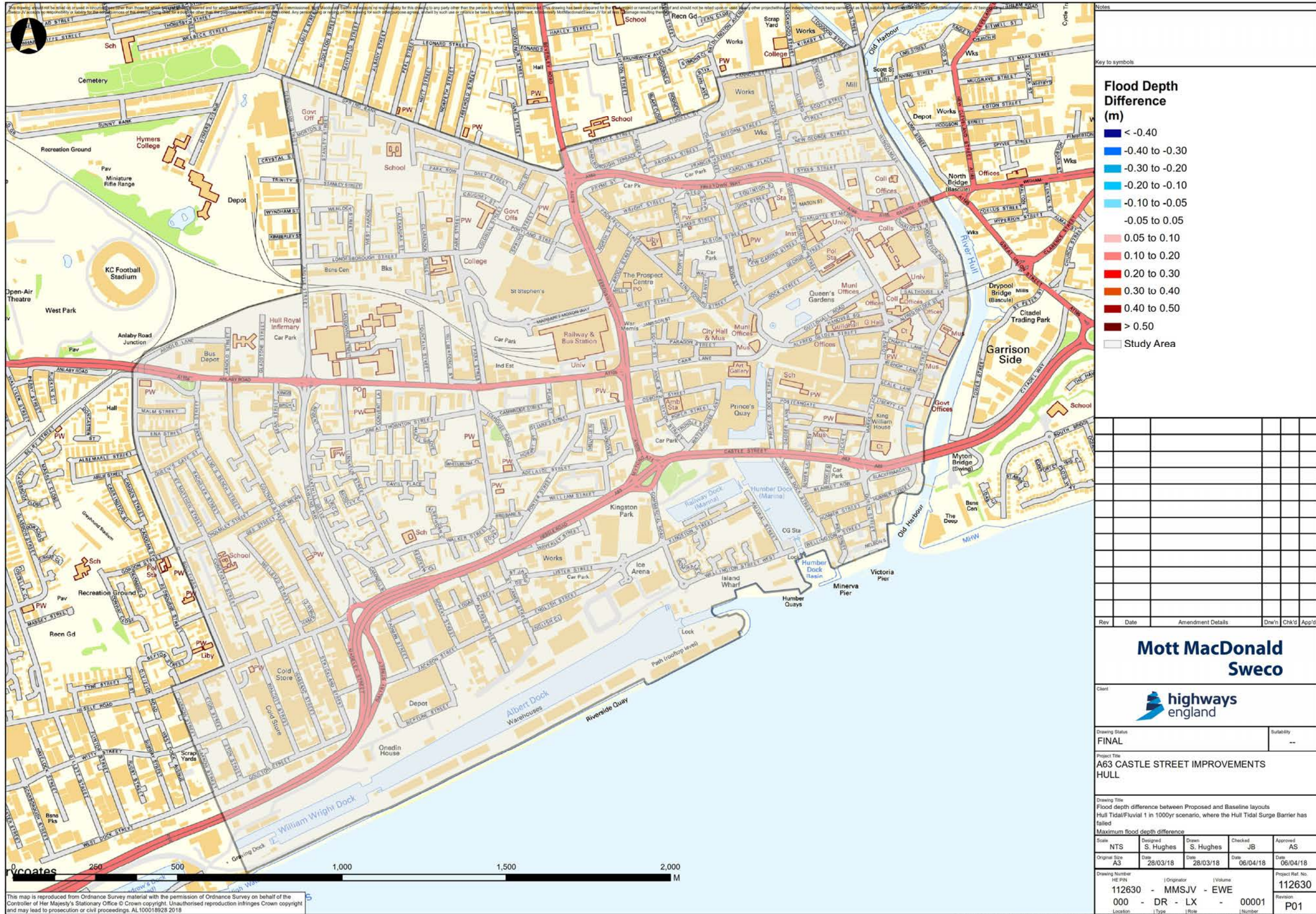
Figure 13.56 1 in 1,000-year River Hull tidal / fluvial flooding maximum flood depth difference (Hull Tidal Surge Barrier open)
